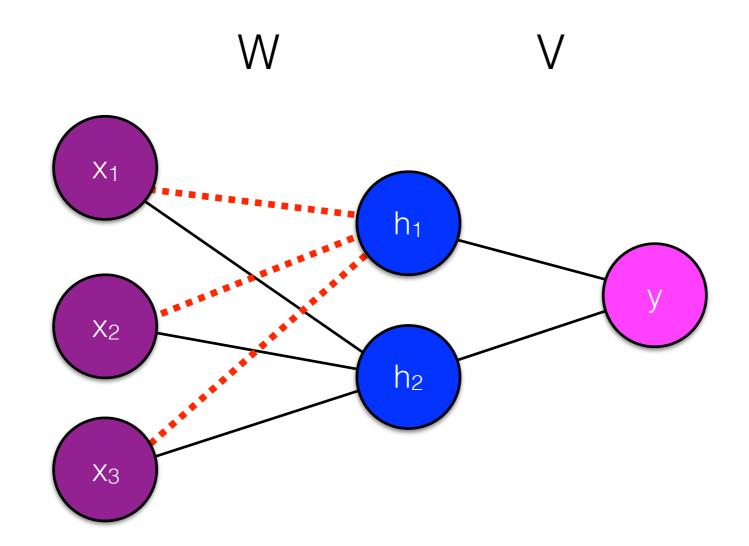
$$\hat{y} = V_1 \underbrace{\left(\sigma\left(\sum_{i=1}^F x_i W_{i,1}\right)\right)}_{h_1} + V_2 \underbrace{\left(\sigma\left(\sum_{i=1}^F x_i W_{i,2}\right)\right)}_{h_2}$$
