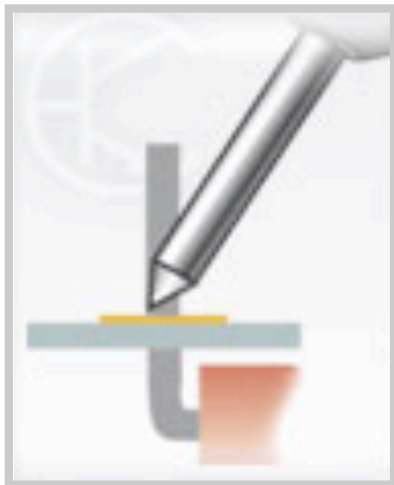
1 Heat the joint, not the solder
