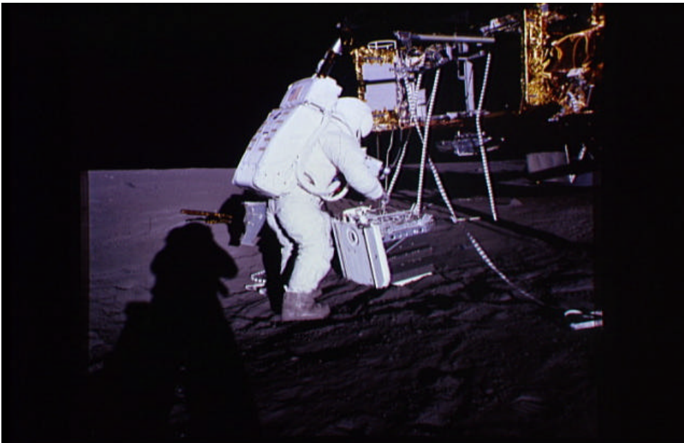
Figure 18. NASA picture AS12-46- 6785: Al has placed the RTG package on the ground. Note the cooling fins on the RTG. Note the pull rings on the edge closest to Al. These pull rings are used to release "pip pins" with which some pieces of equipment are attached to the RTG pallet. The light-colored piece of gear that is attached to the part of the RTG pallet that is on top in this picture is the SIDE (Suprathermal Ion Detection Experiment). Note the deployment rail and pulleys extending out from the SEQ bay above the upper ends of the lanyards. The distinctive ring-shaped top of the fuel cask can be seen behind the lefthand SEQ bay door. Note the saddlebag on Al's left hip and note, also, that Pete's shadow shows that he is wearing one too.
