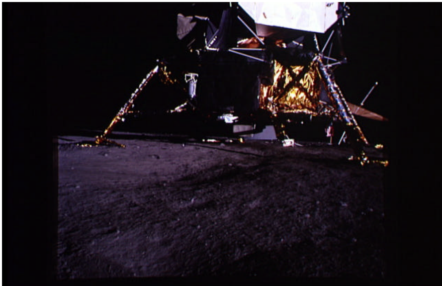
Figure 14. Showing the southeast quadrant of the LM. The upright cylinder stowed against the LM just to the left of the SEQ (Scientific Equipment) bay is the cask holding the plutonium fuel element that will fuel the Radioisotopic Thermoelectric Generator (RTG) that will be deployed as part of the ALSEP (Apollo Lunar Surface Experiment Package).
