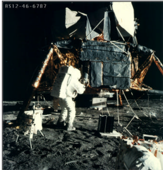
Figure 20. At about 116:43:02, Al is using the dome removal tool. The fuel element is at about 1500 degrees and even the dome is hot enough that Al wants to avoid touching it. The RTG is the dark object at his right. The Handtool Carrier (HTC) is at his left with the hammer sticking up out of the corner nearest the camera. The foreground object at the lower right is ALSEP Package 1, the one that Pete offloaded. Note that Pete has removed the SIDE from the RTG pallet. It was attached on the side which is now facing the right edge of the picture. Pete took the SIDE off the RTG package at 116:41:29 (see 1.5.14). Note that the Universal Handling Tool (UHT) is sticking out of the right side of the base of the RTG pallet. Pete used the UHT to release a Boyd Bolt that was holding the SIDE on.
