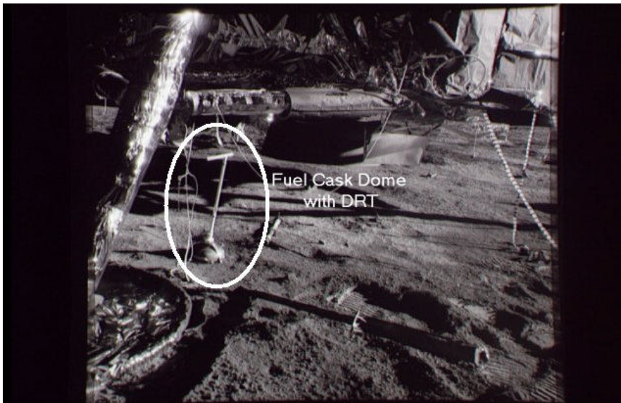
Figure 22. 132:00:36 AI took this view under the engine bell to show a rock that remained in place. Note the fuel cask dome at the left of center, with the dome removal tool still in place. The fuel cask is at the upper right.
