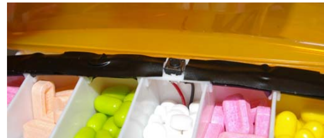
Figure 4 Push button switch activates when opened or closed.
