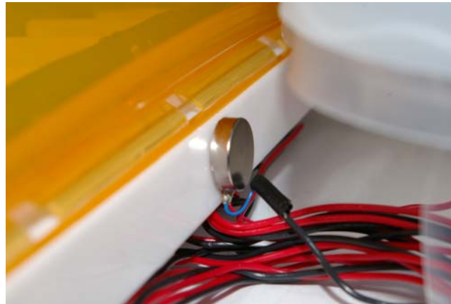
Figure 5. Vibration motor attached in back of pill box.
