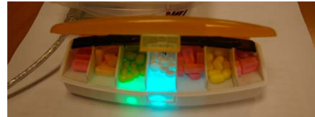
Figure 3. LEDs illuminate respective medication compartments.
