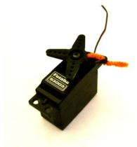
2. Connect the servo motor to your Arduino.
