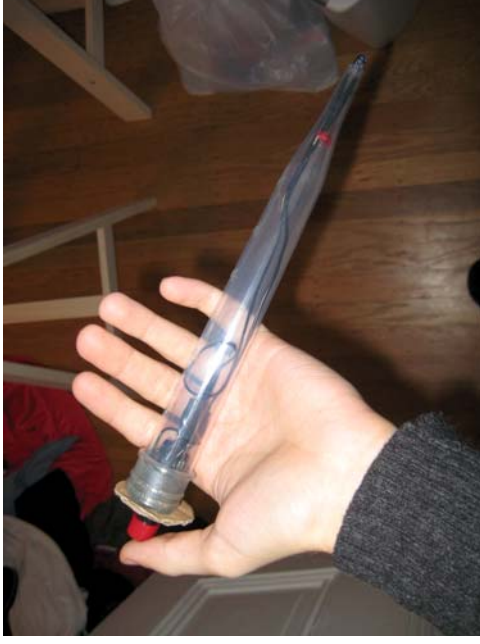
figure 2. The dropper tool, used for selecting colors on the screen interface (fig. 1). Pushing the button activates color selection – this implementation is discussed later.
