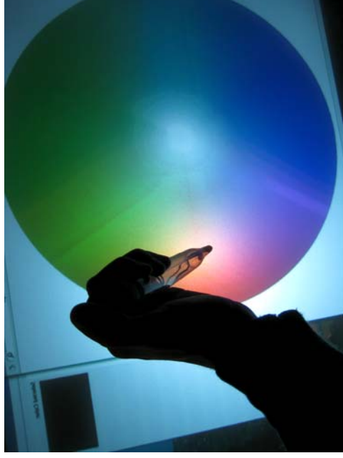
figure 3. The dropper tool in use, selecting a color. Note the button being pushed to signify a color choice.
