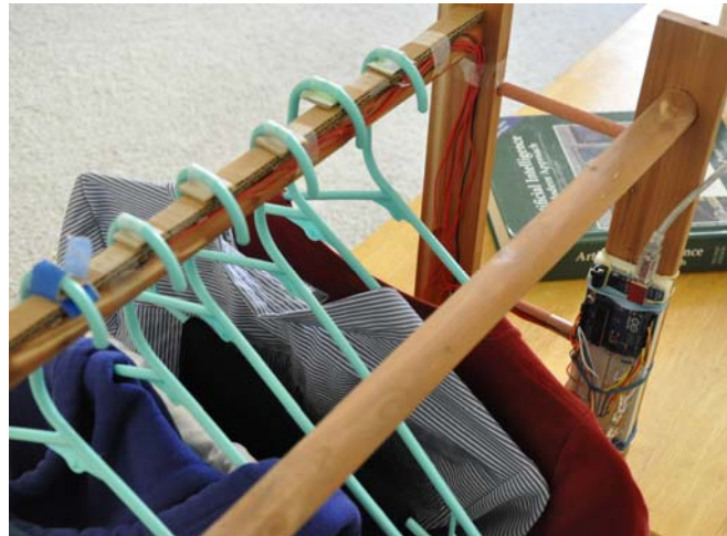
figure 4. Each hanger covers a photocell which is connected to the Arduino board which is connected to a laptop displaying the mirror
