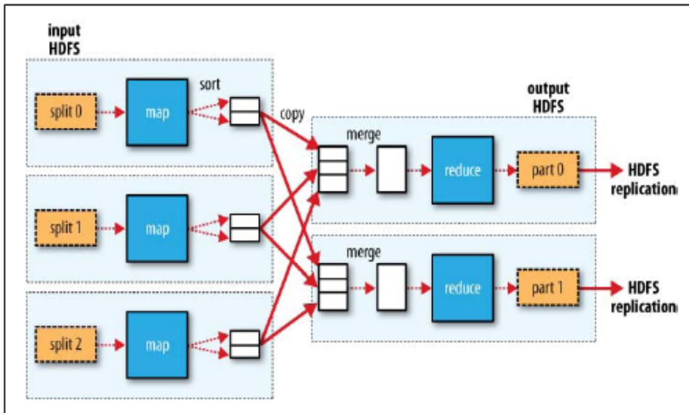
Figure 2-3. MapReduce data flow with multiple reduce tasks
