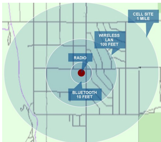
Image 1. Cognitive Radio Systems: One radio dynamically shifts to different types of service (Fette, 2003).
