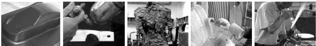
Figure 3. Physical model-making works 3-1.thermoforming modeling, 3-2.spray coloring, 3-3.clay modeling, 3-4.wood carving, 3-5.glass craft (from left to right)
