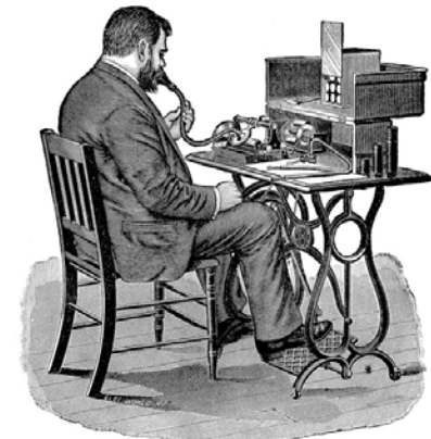
Fig. 2.—Graphophone, 1887, as Used in Dictating a Dictation and for Transcribing.
