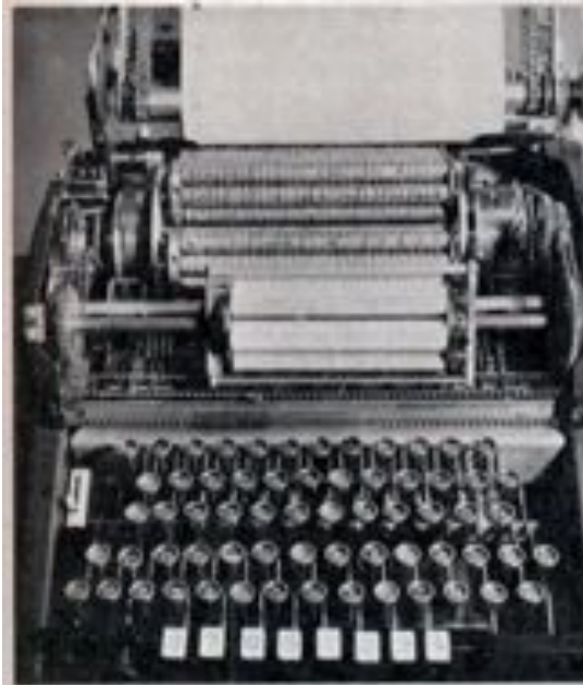
Chinese Typewriter has 72 keys and 576 characters. You press two keys at the same time, one for the top part of a character and one for the bottom. This puts eight words into printing position. You select and print the word you want by pressing one of the eight white keys.
