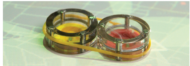
Figure 7: A rubber band used as a mechanical constraint to keep two pucks in close physical proximity.
