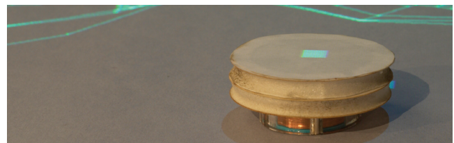
Figure 12: The object placed on top of the puck is filled with sand, preventing the computer from moving the puck autonomously.
