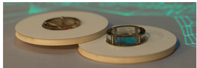
Figure 10: Collars at differing heights can yield different minimum distance constraints for different combinations of pucks.
