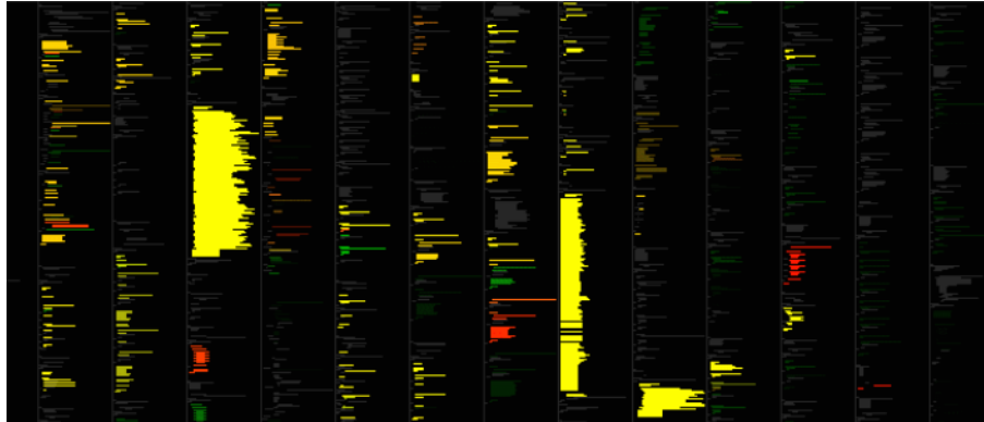
Figure 9: Tarantula visualizes fault localization information by setting the statements' background color according to their likelihood of containing a bug.
