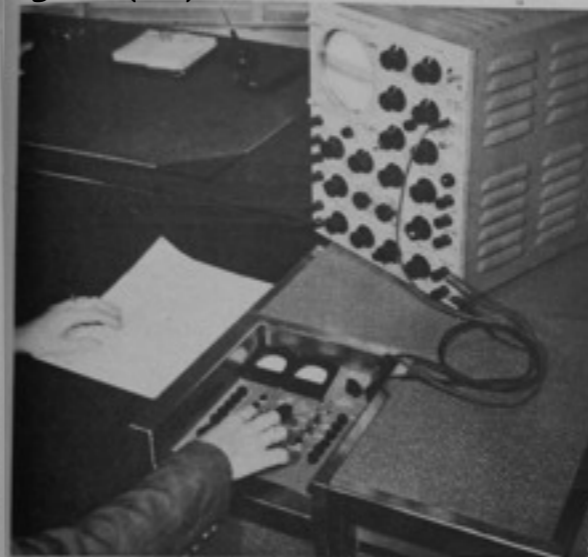
Under the operator's hand is the desk-sized computer called MADDIDA (Mad Ida), for MAGnetic Drum Digital Differential Analyzer, developed by Northrop Aircraft and now in production. Mainly for engineering, it pioneers compact features for general use.
